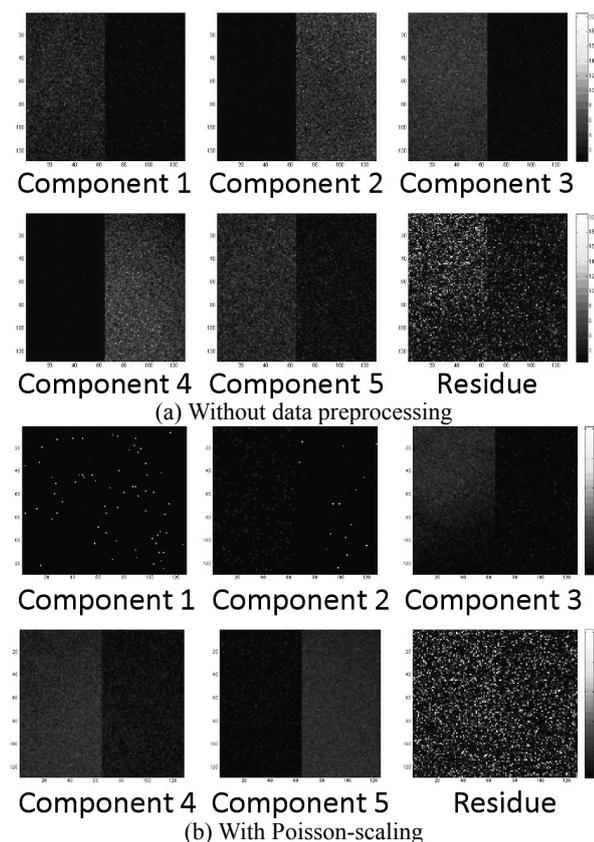
Fig. 2. Secondary ion images of the components extracted by MCR when the number of components is assumed to be five. The left half of each figure is from TOF-SIMS data of the lysozyme-immobilized sample and the other half is from those of the reference sample (ITO-coated glass substrate). Field of view is 120  $\mu\text{m}$ .
