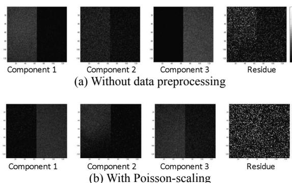
Fig. 1. Secondary ion images of the components extracted by MCR when the number of components is assumed to be three. The left half of each figure is from TOF-SIMS data of the lysozyme-immobilized sample and the other half is from those of the reference sample (glutaraldehyde-activated aminosilanized ITO-coated glass substrate). Field of view is 120  $\mu\text{m}$ .
