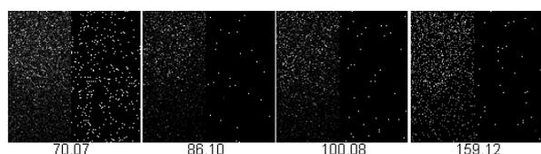
Fig. 4. Secondary ion images of the protein-related peaks, m/z 70, 86, 100 and 159. The left half of each figure shows the lysozyme-immobilized sample and the right one shows the control sample.
