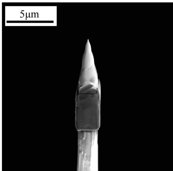
Fig. 3. Specimens which was needle-shaped by the annular milling method.
