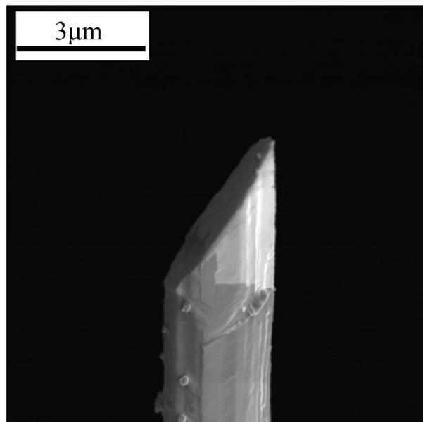
Fig. 4. Specimens which was ruptured by detachment of a Si chip from a W base needle: method (a).
