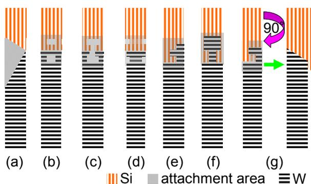
Fig. 1. Schematic images of specimens prepared by attachment methods (a)-(g).
