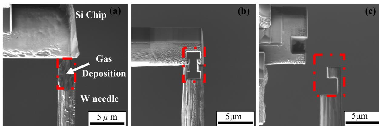
Fig. 2. (a) Specimens which was prepared using welding method (a). (b) Specimens which was prepared using physical strength of C deposition :method (c). (c) Specimens which was prepared using physical strength of joint between sample and base needle :method (g).
