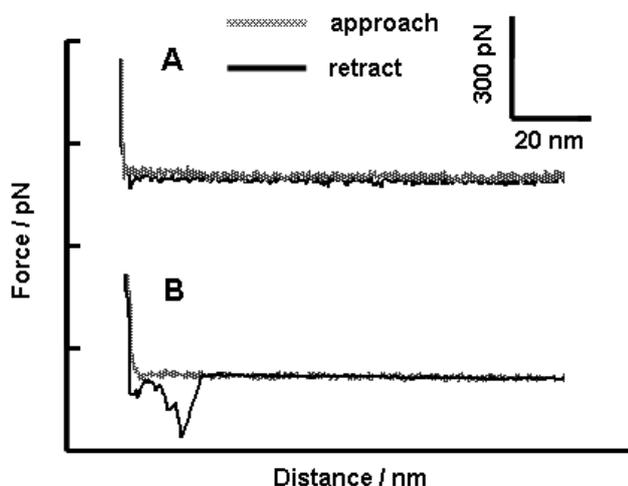
Fig.4. Typical AFM force curves obtained from (A) OEG-terminated, and (B) Man-terminated regions.
