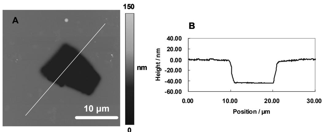
Fig.3. (A) AFM topographic image of the Man- and OEG-terminated pattern substrate. The higher and lower parts were the Man- and OEG-terminated regions, respectively. (B) Cross-section profile of the patterned substrate along the white line shown in (A).
