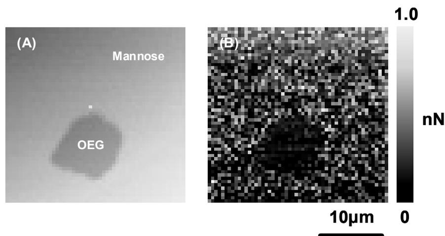
Fig.6. (A) AFM topological image and (B) adhesion force image of the Man- and OEG-terminated pattern substrate obtained with a *ConA*-modified tip.
