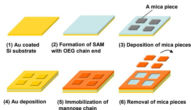
Fig.2. Schematic diagram of fabrication of patterned substrate using mica pieces.
