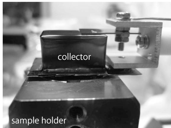
Fig. 2(a) The outer view of the secondary electron collector located on the sample holder.
