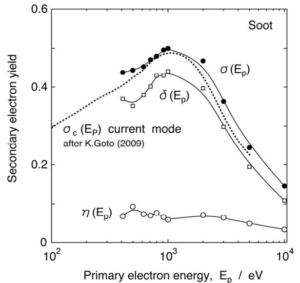
Fig. 5 The secondary electron yields of soot measured by the charge amplification method as a function of the primary electron energy in comparison with that measured by the conventional current-mode method indicated by dashed line.  $\sigma(E_p)$  denotes the total secondary electron yield,  $\delta(E_p)$  the true secondary electron yield, and  $\eta(E_p)$  the backscattering electron yield, respectively. Each data point was measured with the primary electron charge of  $\sim 1$  pC.
