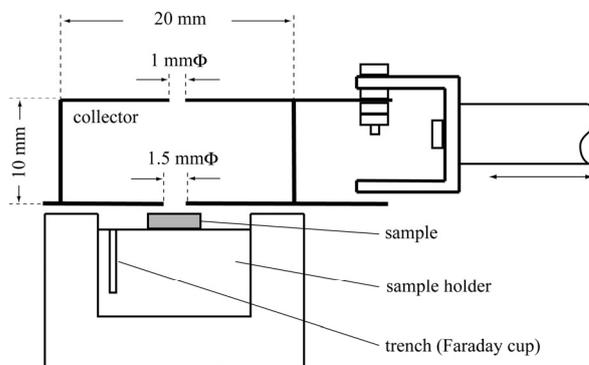
Fig. 2(b) The schematic drawing of the secondary electron collector.
