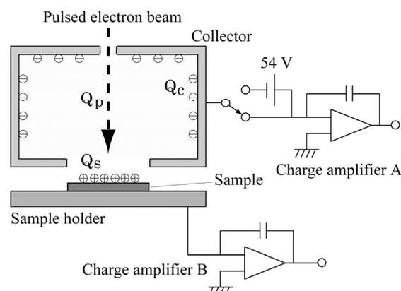
Fig. 1 Schematic of the measurement of SEY of insulators by the charge amplification method.
