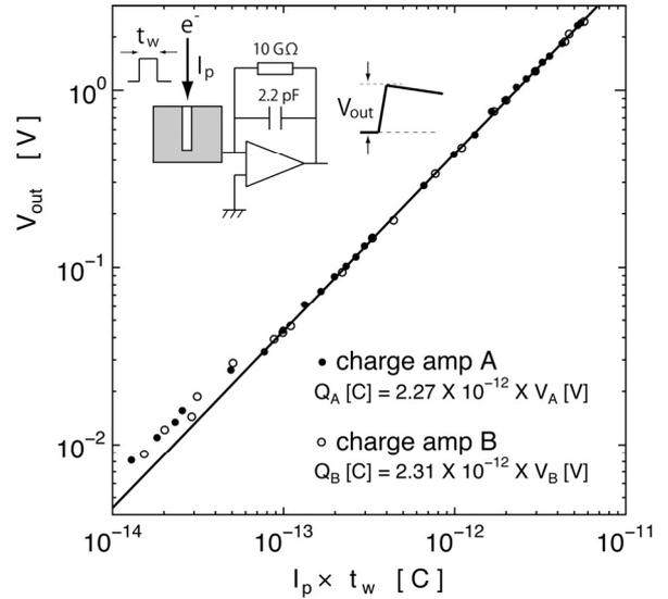
Fig. 4 The input/output characteristics of charge amplifiers A and B. The primary electron energy  $E_p$  was 2 keV, and the pulse width  $t_w$  was 1 ms. The input charge was determined by  $I_p t_w$ , where  $I_p$  is the primary electron beam current measured by the trench on the sample holder.
