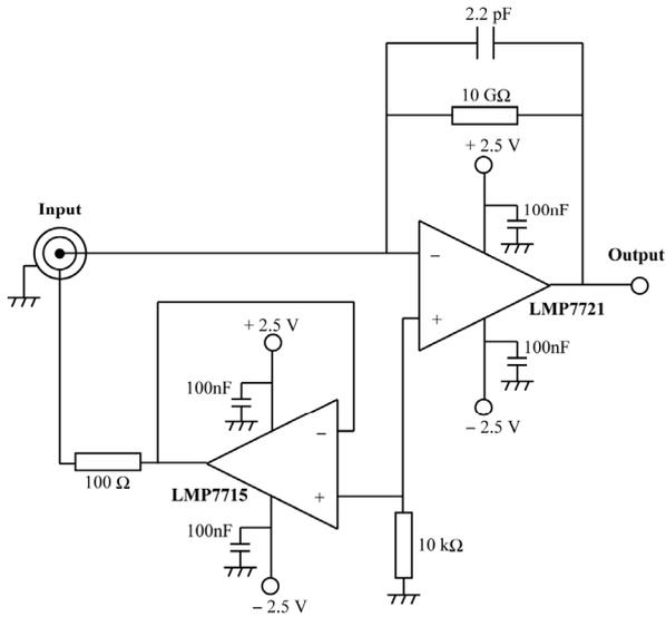
Fig. 3 The electric circuit diagram of the charge amplifier. The input bias current of the LMP7721 operational amplifier is 3 fA.
